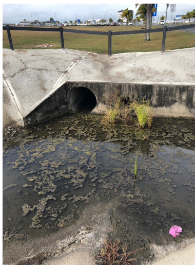
Sediment Sample SS01 - Silt, brown, saturated, low plasticity, organic odour, no sheen
